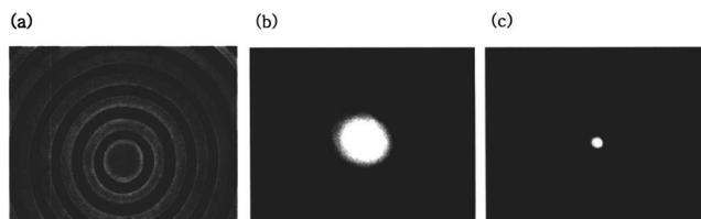
FIG. 3. (a) Optical micrograph of a patterned FTL having a focal length of 1 mm. (b) CCD image of collimated 632.8 nm light at focal plane (without patterned FTL). (c) CCD image of collimated 632.8 nm light at focal plane (with patterned FTL).
