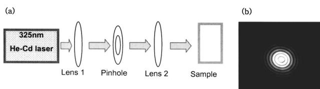
FIG. 2. (a) Schematic configuration for PHD patterns. (b) CCD image of PHD patterns.
