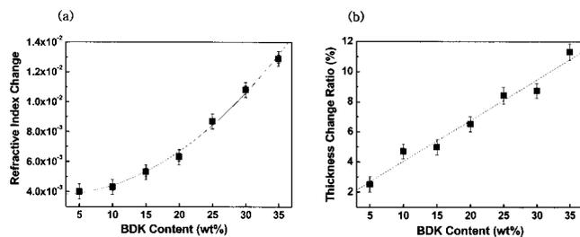
FIG. 1. Refractive index changes (a) and thickness changes (b) in UV exposed SGH film as a function of BDK content.
