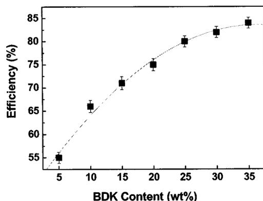
FIG. 4. Diffraction efficiency of FTL as a function of BDK content.
