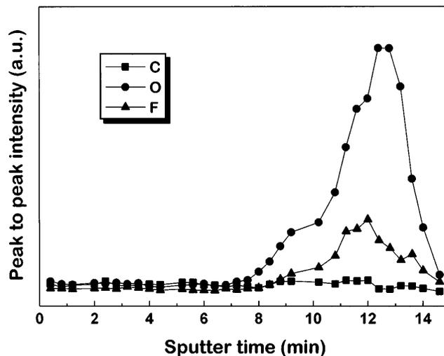
FIG. 5. AES depth profile for  $\text{SiN}_x$ (150 nm)/ $\text{SiN}_x : \text{F}$ (90 nm)/Si structure *in situ* deposited at 250 mTorr, 250 W, 300 °C, and  $\text{SiH}_4 : \text{N}_2 : (\text{NF}_3) : \text{Ar} = 2 : 15 : (1.5) : 150$  (sccm).
