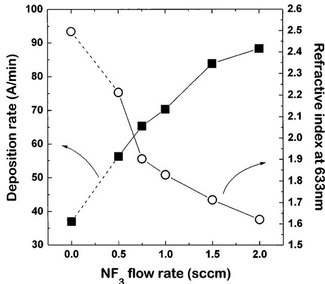
FIG. 6. Effect of  $\text{NF}_3$  flow rate on the deposition rate and refractive index of fluorinated silicon nitride film [250 mTorr, 250 W, 300 °C, and  $\text{SiH}_4 : \text{N}_2 : \text{Ar} = 2 : 15 : 150$  (sccm)].
