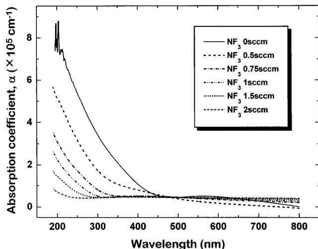
FIG. 7. Effect of  $\text{NF}_3$  flow rate on the absorption coefficient as a function of wavelength of fluorinated silicon nitride film [fused silica substrate, 250 mTorr, 250 W, 250 °C, and  $\text{SiH}_4:\text{N}_2:\text{Ar} = 2:15:150$  (sccm)].
