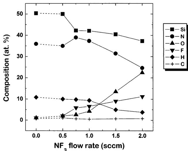
FIG. 3. Composition variation with the  $\text{NF}_3$  flow rate of fluorinated silicon nitride film using ERD-TOF [250 mTorr, 250 W, 300 °C, and  $\text{SiH}_4 : \text{N}_2 : \text{Ar} = 2 : 15 : 150$  (sccm)].
