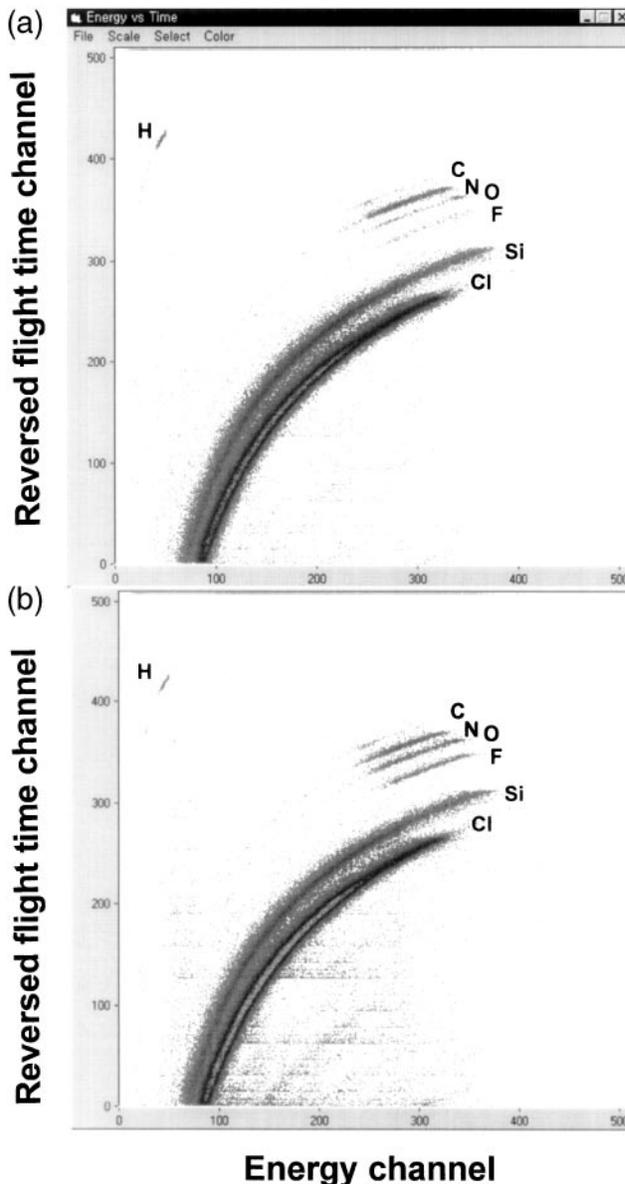
FIG. 2. Energy versus time spectra by ERD-TOF of fluorinated silicon nitride films deposited at 250 mTorr, 250 W, 300 °C,  $\text{SiH}_4\text{:N}_2\text{:Ar} = 2\text{:}15\text{:}150$  (sccm) and  $\text{NF}_3$  flow rates of (a) 0.5 sccm and (b) 1.5 sccm.
