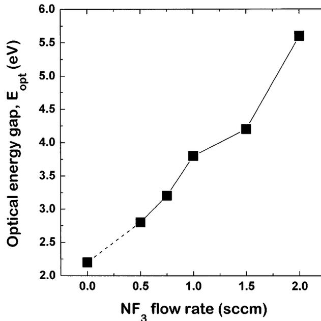
FIG. 8. Effect of  $\text{NF}_3$  flow rate on the optical energy gap of fluorinated silicon nitride film [fused silica substrate, 250 mTorr, 250 W, 250 °C, and  $\text{SiH}_4:\text{N}_2:\text{Ar} = 2:15:150$  (sccm)].
