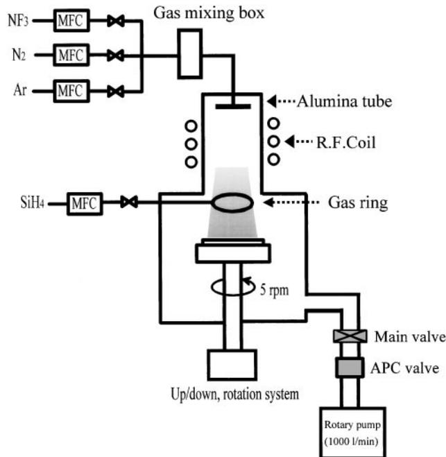
FIG. 1. A schematic diagram of ICP enhanced CVD system.
