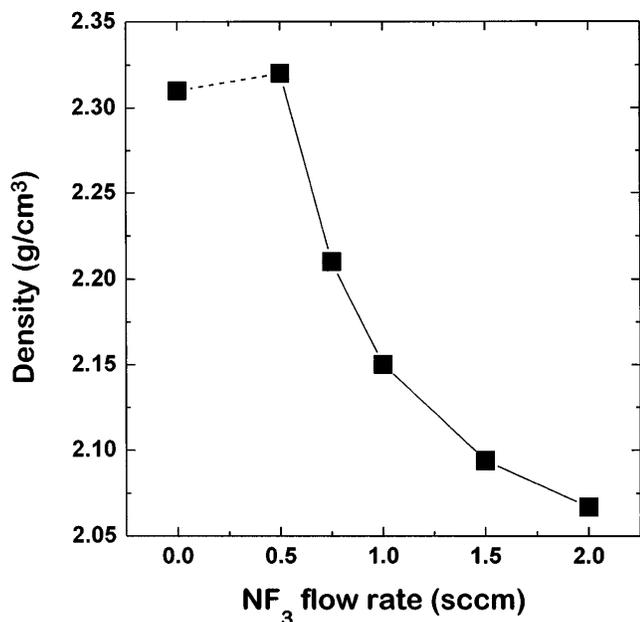
FIG. 4. Film density variation with the  $\text{NF}_3$  flow rate of fluorinated silicon nitride film [250 mTorr, 250 W, 300 °C, and  $\text{SiH}_4 : \text{N}_2 : \text{Ar} = 2 : 15 : 150$  (sccm)].
